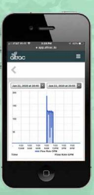
THE PUMP CONTROL SCREEN PROVIDES CONFIRMATION THE PUMP IS ON, A 24 HR CHART OF SENSOR ACTIVITY, AND CURRENT SENSOR VALUE.
