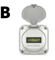
**B:** The default calibration for the Altrac is 100 gallons per pulse. Check your flow meter settings to determine the proper gallons per pulse calibration value. You may need to use a magnet to view the menu. If the value is differs from 100 gallons per pulse contact Altrac to update your Flow Meter Station.
