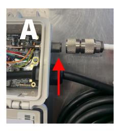
A: Remove the plastic protective cap on the COAX connector and screw the antenna cable onto the COAX connector. The connector should be snug.
