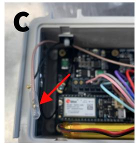
C: Remove the clear protector from the COAX antenna cable.
