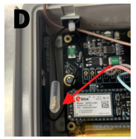
D: Place the clear protector on the TAOGLASS antenna cable. This prevents the metal tip from shortcircuiting other electronics.
