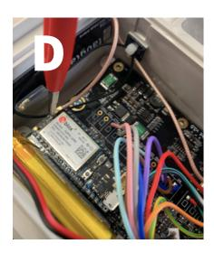
D: Attach the COAX antenna cable to the cellular modem by aligning the connector over the brass nipple and gently pressing down directly over the top of the connector.
