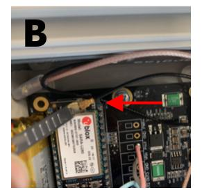
B: You need to switch the antenna cable so the COAX sends the cellular signal to our modem. Start by finding the internal antenna (TAOGLASS Black Rectangle), follow the wire, and remove the connector from the cellular modem by pulling up
