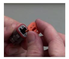
4. Once all contacts are in place, insert wedge. The wedge will snap into place.
