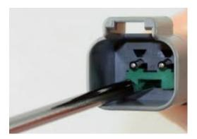
4. Once all contacts are in place, insert wedge. The wedge will snap into place.
