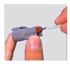
3. Push contact straight into connector grommet until a click is felt. A slight tug will confirm that it is locked in place.
