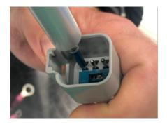
2. Apply pressure toward contact until slide aligns with indicator line. **Contact should** remain in place.
